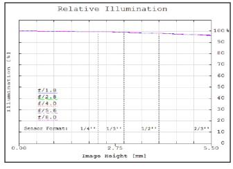
Figure 2: Relative illumination (center to corner)
