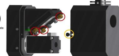
Figure 2. Disassembly of EO Attenuator. Adjustment microscrews circled in red. To remove the cover loosen two screws on each side of EO Attenuator (marked with yellow circle)
