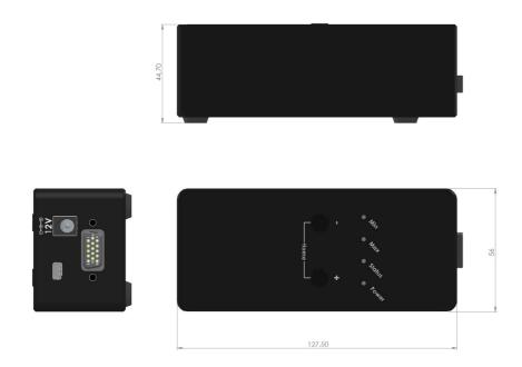
Figure 12. Main dimensions of EO Attenuator controller.
