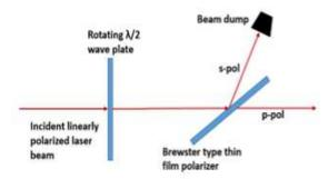
Figure 1. EO Attenuator operation principle. The intensity of the incident beam is varied by means of a  $\mathbb{Z}/2$  phase waveplate and a polarizer.
