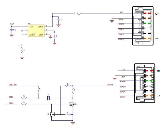
Non-isolated input and output circuit—Board-level
