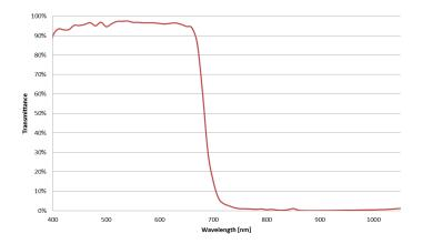
IR filter transmittance graph
