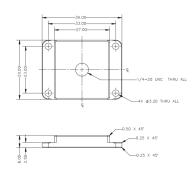
Tripod Adapter Dimensional Diagram Standard Case (ACC-01-0003)
