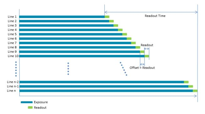
An advantage of a rolling shutter with global reset is a reduction in image artifacts typical of rolling shutters such as skew and wobble. However, because exposure lengthens throughout the frame, there may be a gradual increase in brightness from top to bottom of an image. This gradient can be diminished or even eliminated by using a strobe flash.
